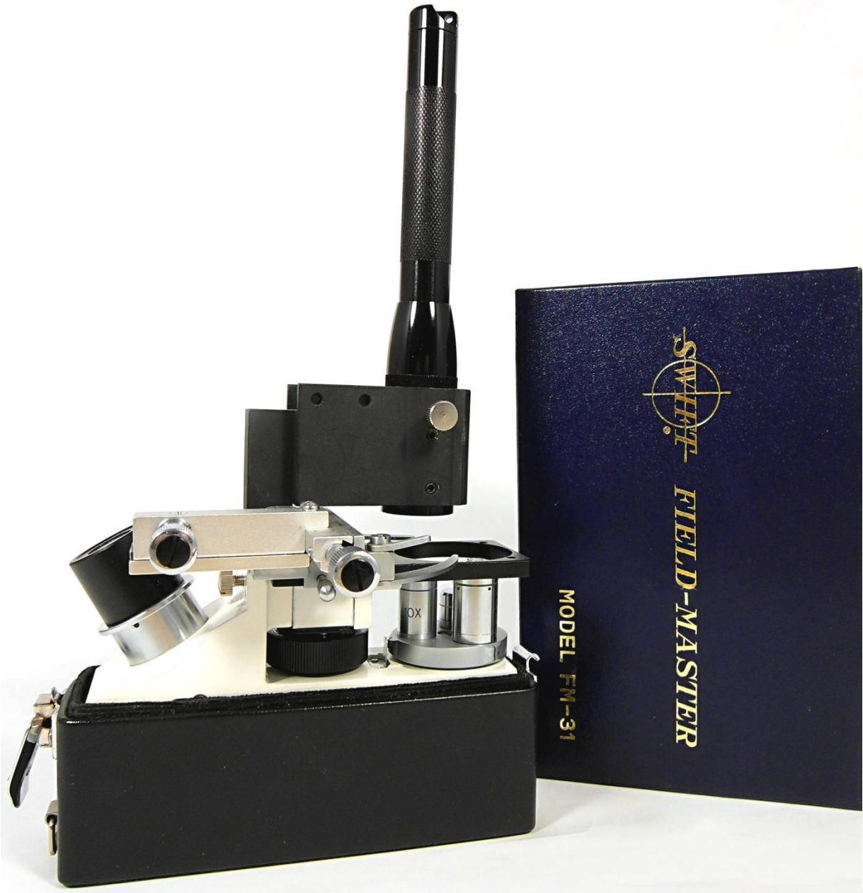
Figure 7. Swift FM-31 with Maglite® illumination c. 1980s
